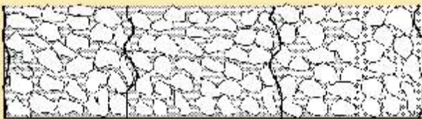
Fig 2 Cell filled Concrete after Compaction
